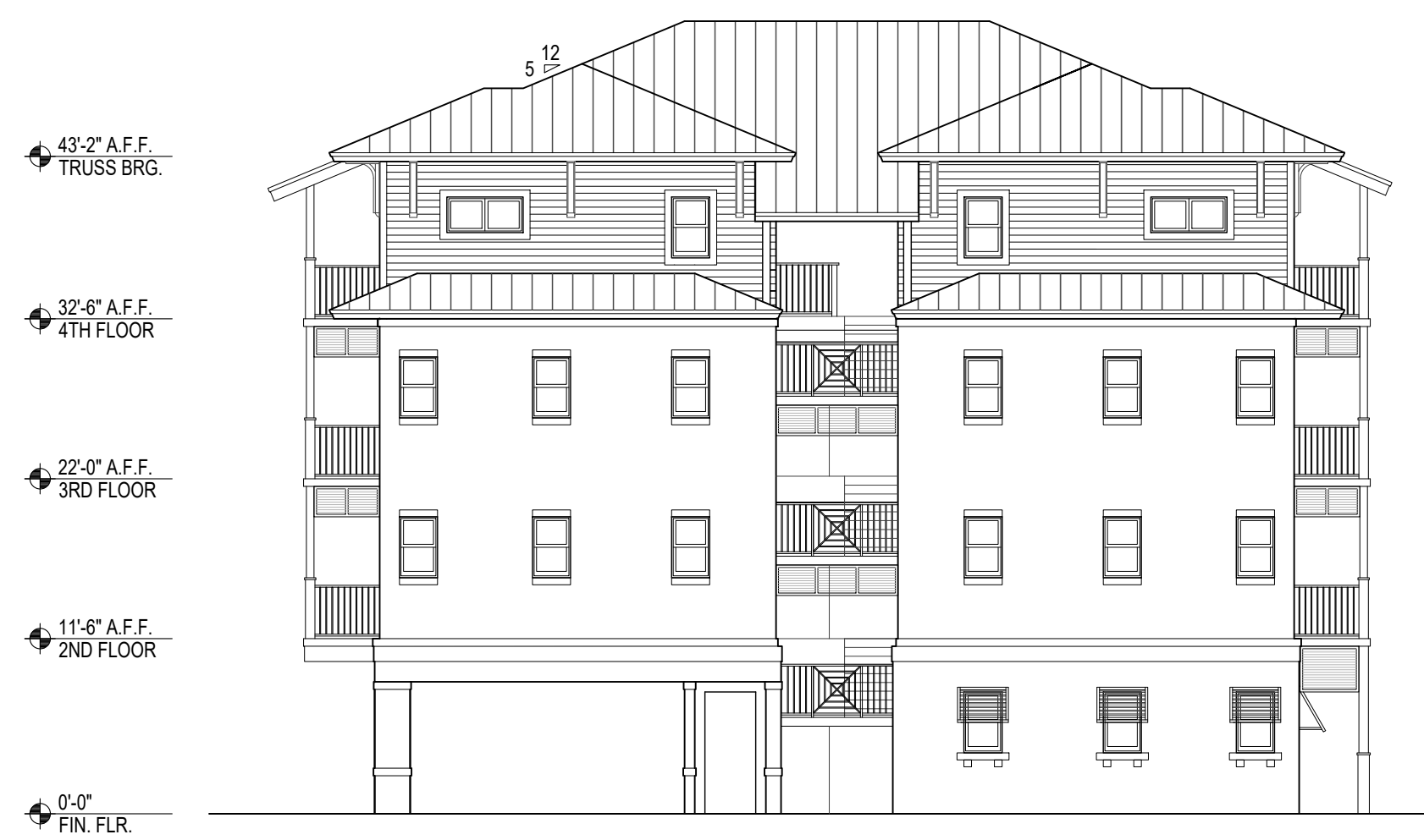
04 SOUTH ELEVATION BUILDINGS 1 & 3 SCALE: 3/32" = 1'-0"
