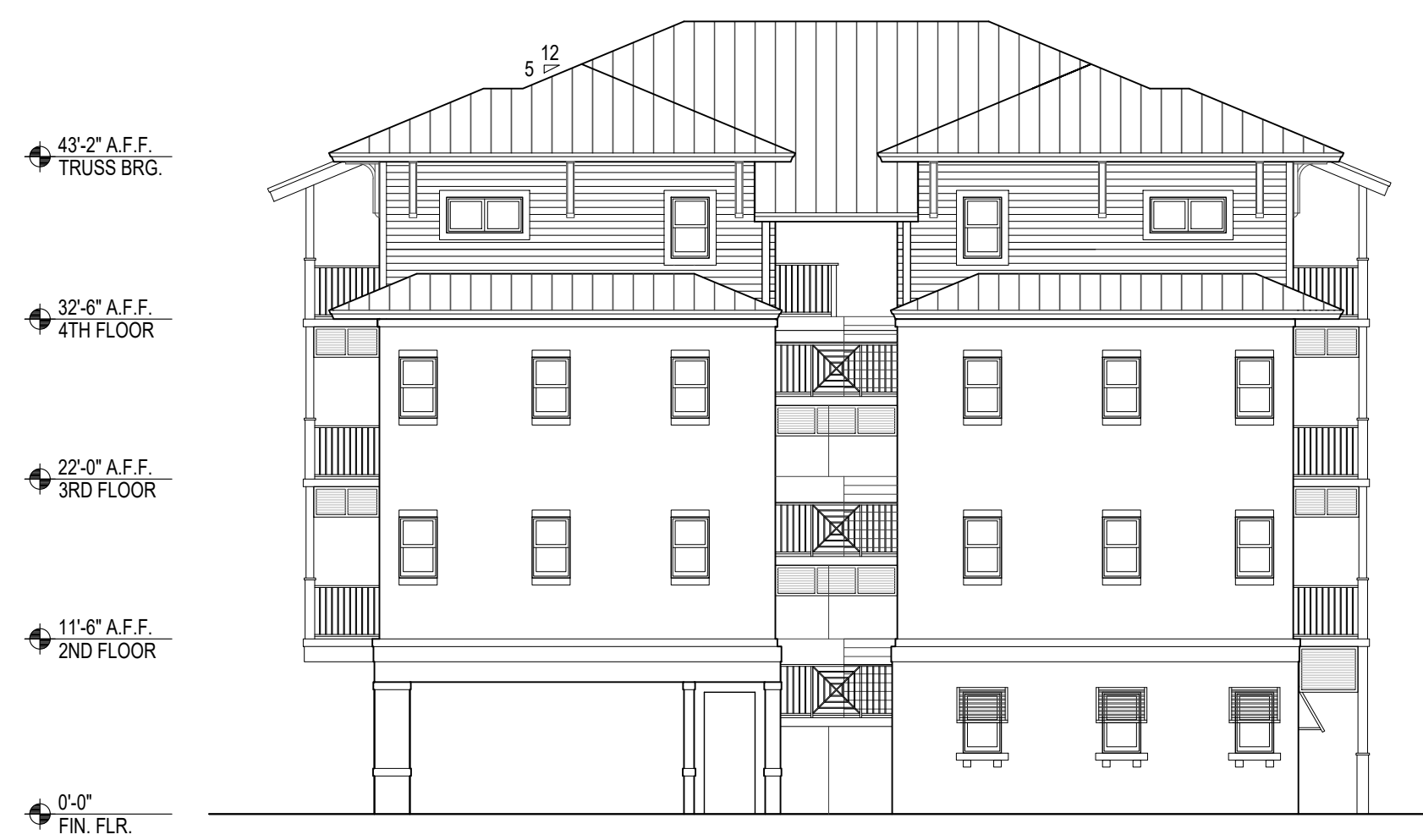
03 NORTH ELEVATION BUILDINGS 2 & 4 SCALE: 3/32" = 1'-0"
