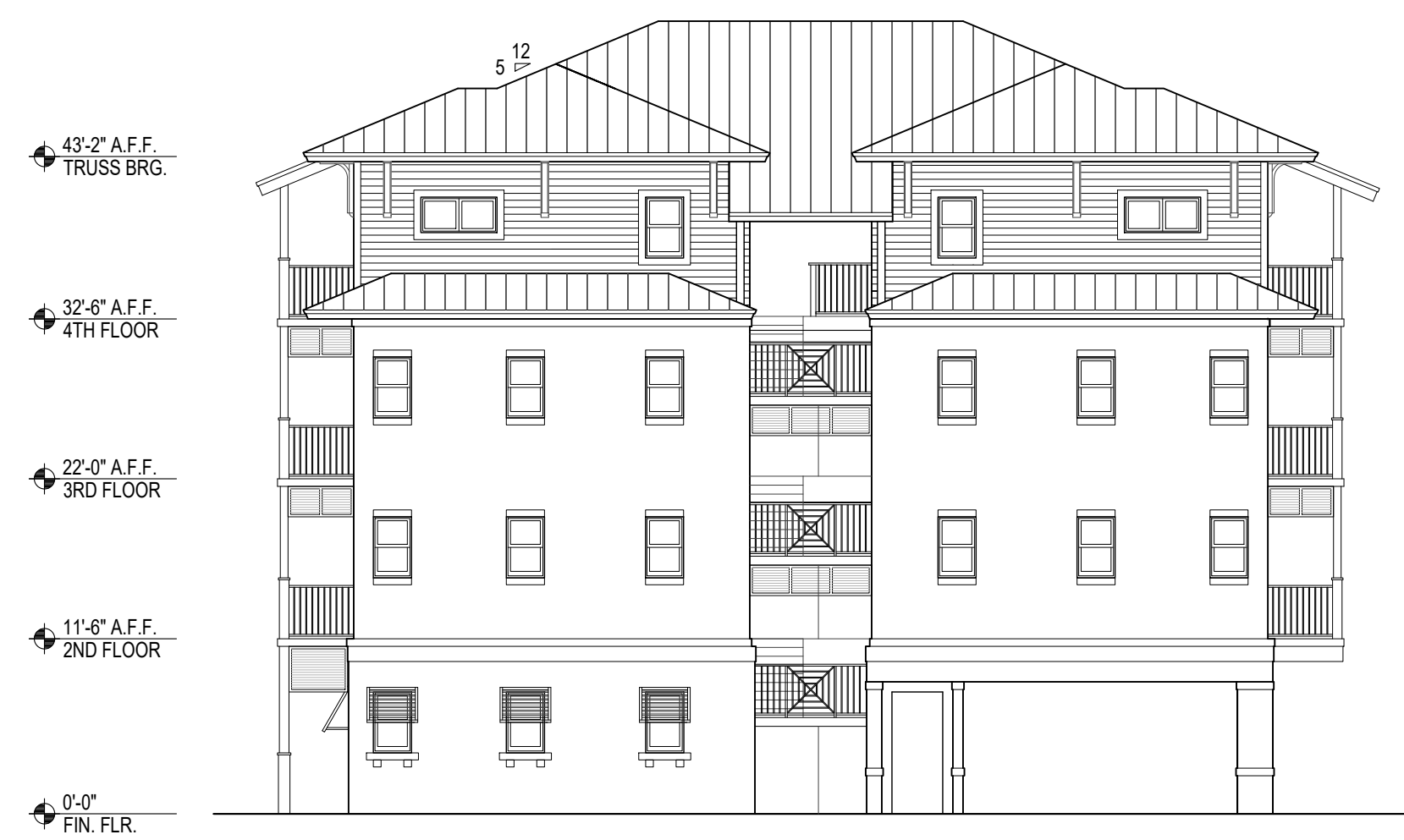
04 SOUTH ELEVATION BUILDINGS 2 & 4 SCALE: 3/32" = 1'-0"
